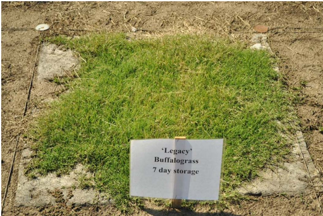
Figure 3. 'Legacy' buffalograss stored for 7 days on TRM prior to establishment. This photo was taken September 22, 2011, after planting on mat July 1, 2011.
