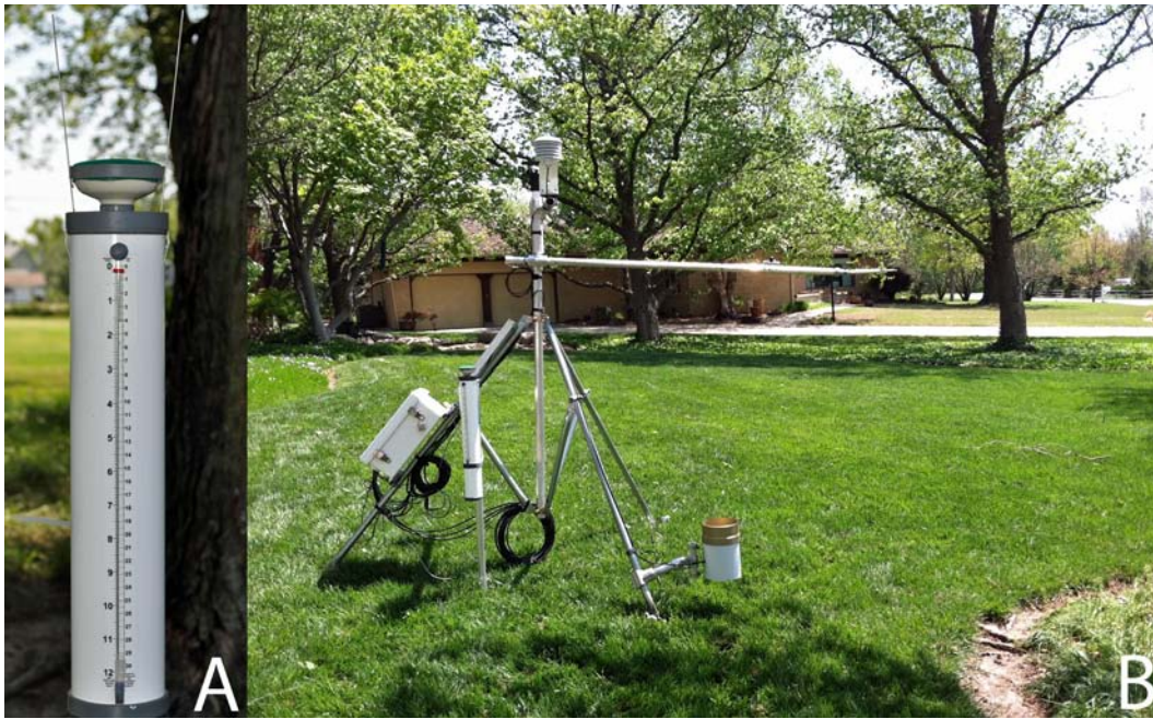
Figure 1. Closeup of an atmometer (A) and a weather station with atmometer (B) collecting data in an urban microclimate.
