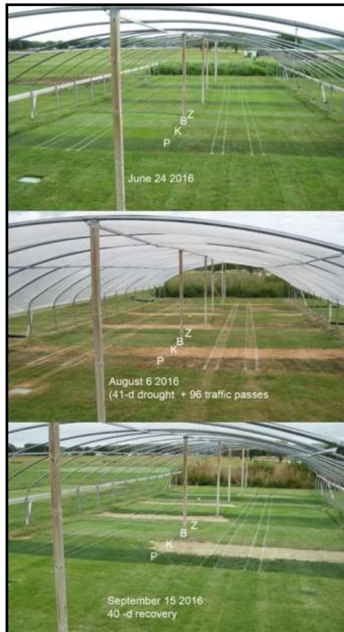
Figure 2. The 2016 study area of zoysiagrass (Z), buffalograss (B), Kentucky bluegrass (K), and perennial ryegrass (P) during the pre-drought (top), at the end of the 41-day drought period (middle), and at the end of the 40-day recovery (bottom). Plots immediately right of the turf species letters are at rough mowing height, while plots immediately left of letters are at fairway mowing height. Traffic passes only occurred inside the white lines.
